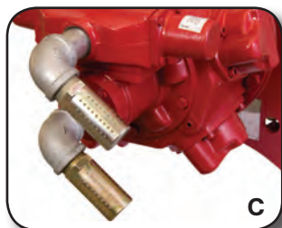
Mufflers help reduce noise during operation.
